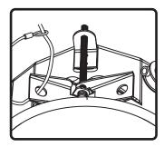
**5.** If required, attach seismic restraint system to hole in clamping arm, then to reinforced structure (safety cable not included).
